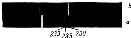
FIG. 2. The U II line 4244.372 Å with components of three isotopes: a --- spectrum of a mixture of three isotopes of uranium, b --- spectrum of natural uranium.
