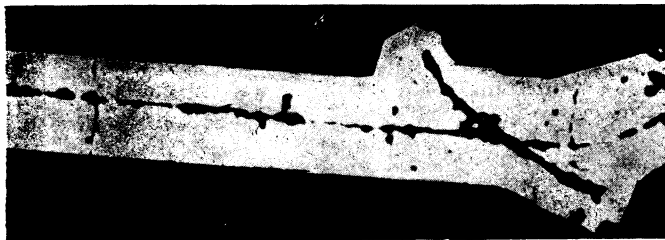
FIG. 7. Fission of the uranium nucleus on capture of a \pi^- meson with emission of an \alpha -particle.
