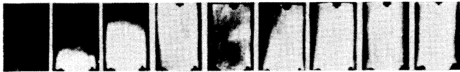
FIG. 6. Photograph of the glass tube beyond the upper electrode of the cylindrical chamber during discharge in deuterium; C = 43 \mu\text{f} , U_0 = 25 \text{ kv} , p_0 = 0.2 \text{ mm Hg} .
