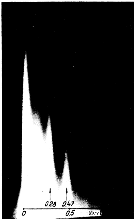
FIG. 7. Spectrum of As. The 0.28 Mev line, not found in the background spectrum, is quite pronounced. The photomultiplier was exposed for 134 millisecc, 4 millisecc after start of neutron pulse. Monitor count – 21,400.
