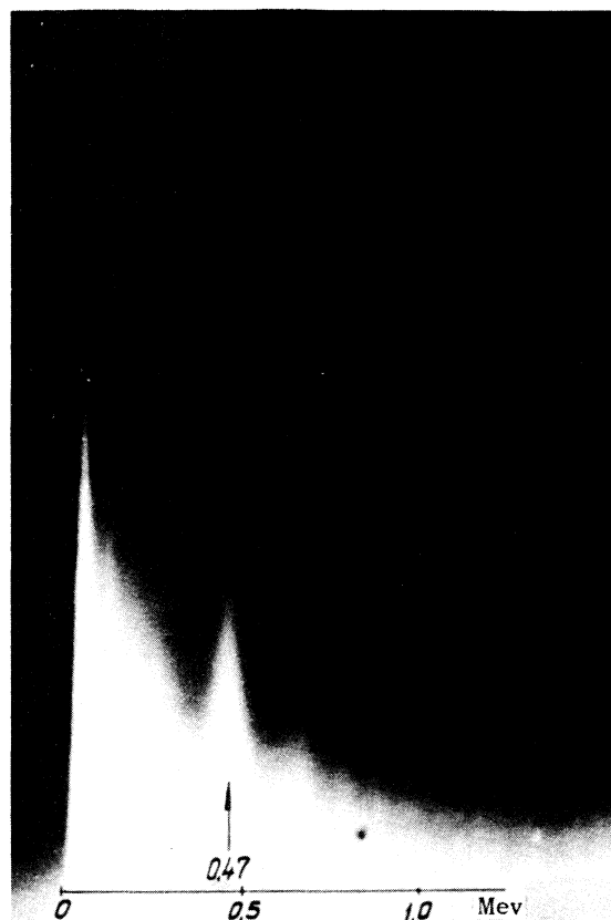
FIG. 3. Background spectrum in absence of sample, obtained by starting the exposure 4 millisecc after start of neutron pulse. Monitor count, 11,600.
