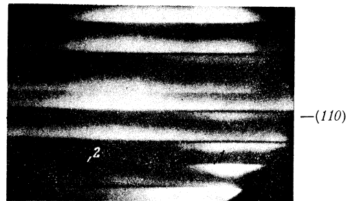
FIG. 3. Transformation of elementary shear traces, 2 into single slip bands, 1 (so called "pencil lines"), after the shear is increased. Crossed prisms ( \times 25 ).
