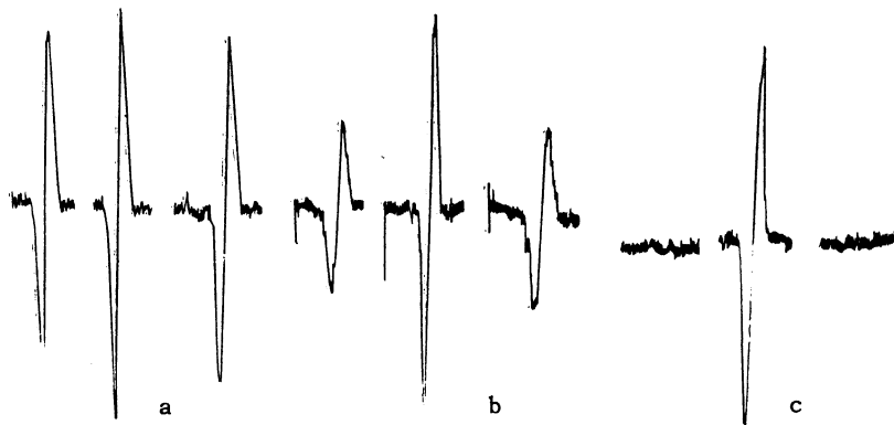
FIG. 1. NMR spectra in various crystals: a) \text{NaNO}_3 , b) \text{NaNO}_3 + 0.5\% \text{AgNO}_3 , c) \text{NaNO}_3 + 2.1\% \text{AgNO}_3 .
