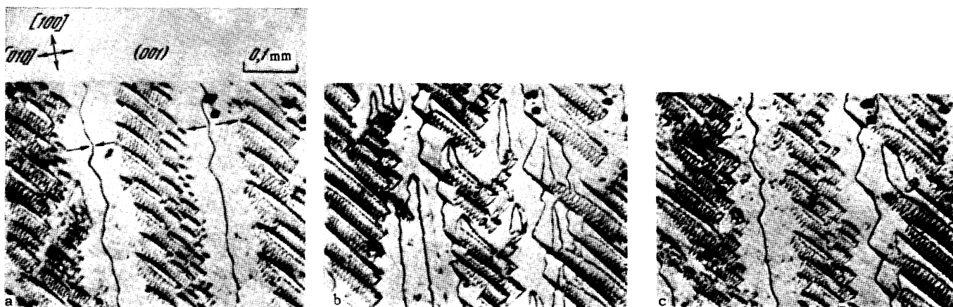
FIG. 3. Powder pattern on a crystal surface approximately parallel to the (001) plane (type B structure): a – after demagnetization, b – after heating to 400°C, c – after re-demagnetization.
