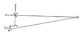
pattern, and M is a system of two mutually perpendicular plane mirrors which can be moved in the direction of the arrow with a controlled speed v.
