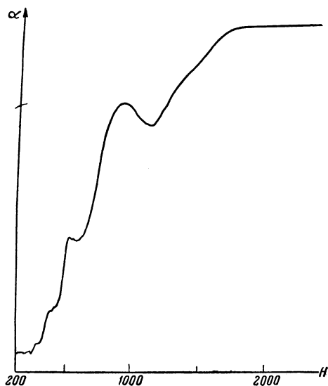
FIG. 7. Record of the dependence of the coefficient of absorption on the magnetic field for q along [100] and H making an angle of 50^\circ with [001] ; \nu = 183 Mc.
