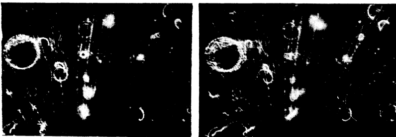
FIG. 9. Stereo photograph of a soft shower in a track spark chamber located in a magnetic field.
