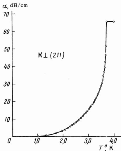
FIG. 1. Temperature dependence of the coefficient of electron absorption of ultrasound of frequency 276 MHz for the orientation of the sound wave vector  $k \perp (211)$  in pure superconducting tin.
