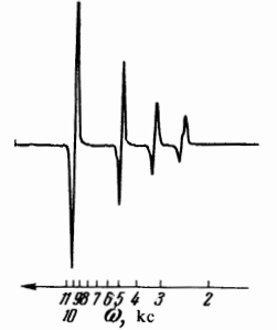
FIG. 1. Magnetic resonance of \text{Cs}^{133} atoms in an effective field at \omega_e/2 = 10 kc.
