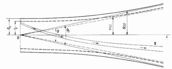
Schematic representation of a non-ideal coherent light beam (fundamental mode).  $\sigma(z)$ -running radius of the beam, defined by (7); S-Poynting vector (9);  $\vartheta_0$  - beam aperture angle,  $\vartheta$  and r(z)-asymptotic angle and radius of the cross section of the single-cavity hyperboloid of revolution (10a).
