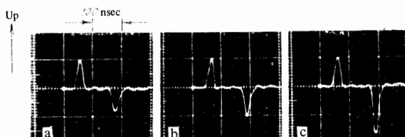
FIG. 2. Oscillograms of the process of absorption saturation for E \perp c : a - P_0 = 250 W/cm 2 , b - P_0 = 6.2 kW/cm 2 , c - P_0 = 22.5 kW/cm 2 .
