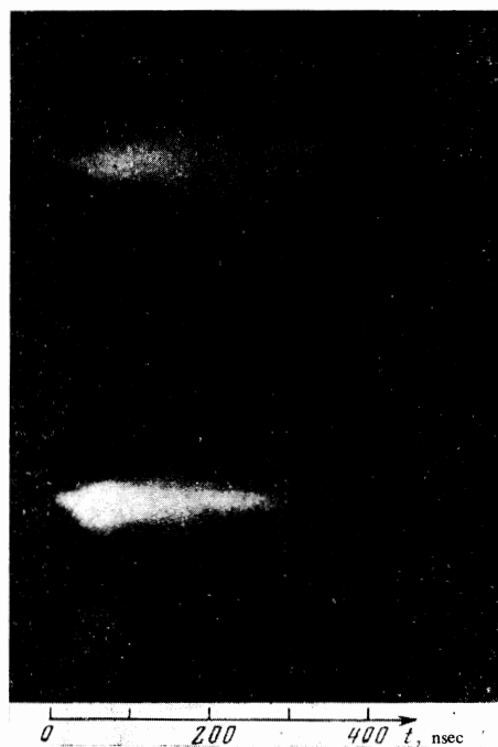
FIG. 5. Photographs of the expansion of the glowing boundary of a plasma along the laser beam (top) and in the perpendicular plane (bottom), B = 0 .
