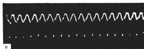
FIG. 4. Emission oscillogram of ruby laser with plane-parallel nonstationary resonator. Sweep duration 50 \mu\text{sec} .
