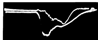
FIG. 7. Oscillograms of beam-current density on the axis of the plasma column (lower trace) and at a distance of 1 cm from the axis (upper trace). \tau_{\text{dev}} \sim 1.0 \mu\text{sec} , W = 40 \text{ keV} , n_0 \sim 8 \times 10^{12} \text{ cm}^{-3} .
