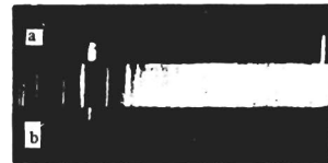
FIG. 5. Scattered spectrum in the direction of the pump (linear polarization): a) scattered spectrum with polarization identical with that of the pump; b) scattered spectrum with reverse polarization.
