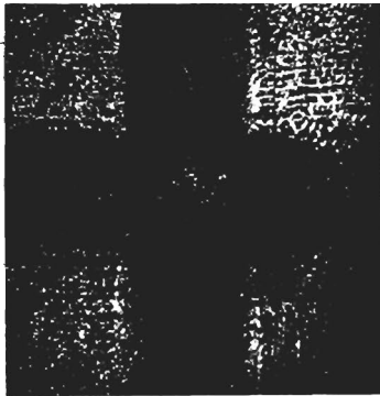
FIG. 7. Acoustic image of object. Frequency 3.2 MHz, layer thickness 40 \mu ( \times 6 ).
