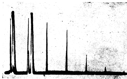
FIG. 2. Polarization echo in an \text{LiNbO}_3:\text{Ni} crystal. The oscillogram shows the microwave and echo pulses; the high intensity of the main signal resulted in the appearance of secondary echo signals.
