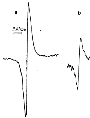
FIG. 2. Plots of EPR signal in Faraday-rotation noise: a— at the edges of the 5896 Å absorption line, b—between the 5896 and 5890 Å lines.
