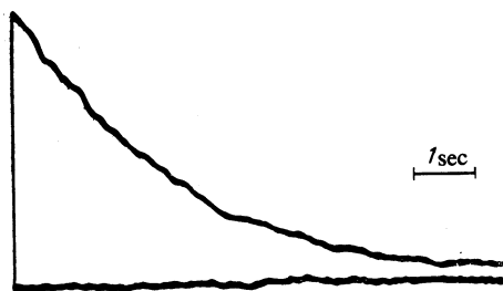
FIG. 5. Spin-lattice relaxation curve obtained in the DRCS at the frequency \Omega / 2\pi = 100 kHz for the protons of distilled water under conditions of steady spin locking at \gamma H_{21} = 3.4 kHz, \theta' = 90^\circ . The bottom curve is the zero line.
