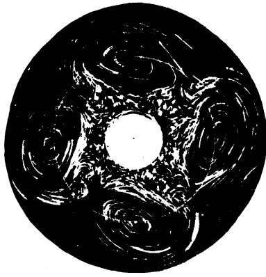
FIG. 8. Example of the generation of steady anticyclonic structures under the conditions of the geometry of Fig. 6.
