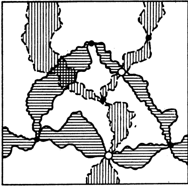
FIG. 2. Schematic of the "backbone" of an infinite cluster. The horizontal and vertical hatching indicates the superlattices for the longitudinal and transverse current, the filled-in circles are the hot points, the wavy lines are the macrobonds at whose intersections (at the bottlenecks) are found the active points (the open circles).
