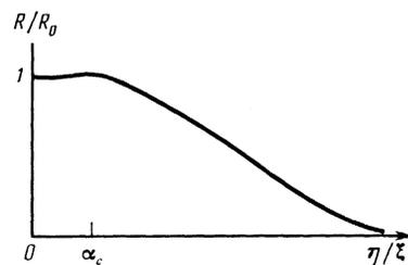
FIG. 3. Dependence of the relative number of reflected particles on the parameter  $\eta/\xi$  for  $|\varepsilon|\eta \ll \xi^2$ , the case  $\eta/\xi \rightarrow 0$  corresponds to the scattering of a linear wave.
