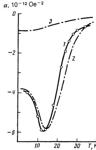
FIG. 2. Temperature dependence of the coefficient  $\alpha$ : 1—experiment; 2—theory,  $A = 22 \text{ cm}^{-1}$ ; 3—theory,  $A = 0$ .
