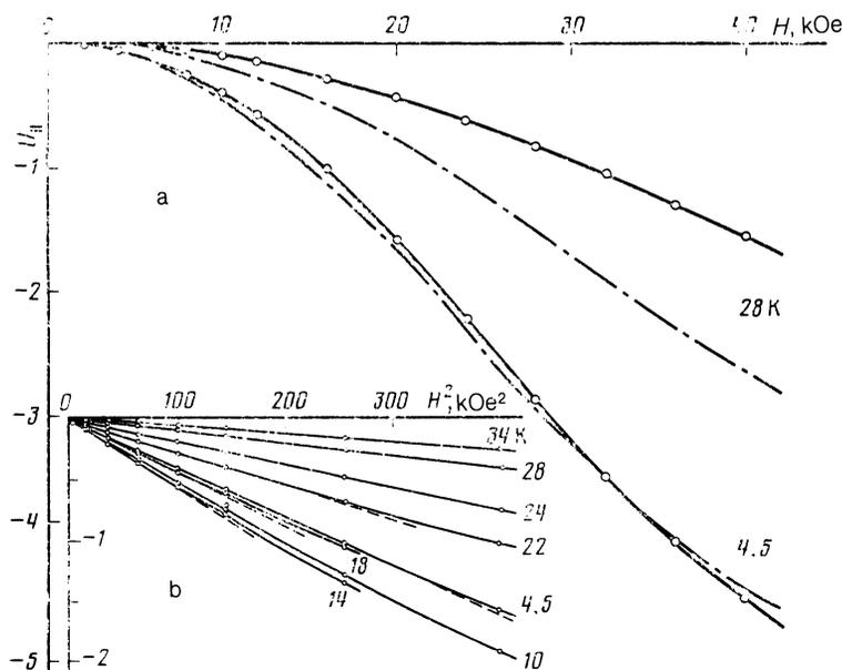
FIG. 1. Isotherms of the longitudinal magnetostriction of single-crystal  $\text{TmPO}_4$  in a magnetic field  $\mathbf{H} \parallel [110]$ : a— $U_{\parallel}(H)$ , b— $U_{\parallel}(H^2)$ ; points—experiment, dash-dot—calculation, dashed—linear extrapolation of the  $U_{\parallel}(H^2)$  dependence in weak field. The ordinate scale is  $10^{-3}$ .
