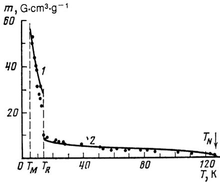
FIG. 1. Temperature dependences of the spontaneous magnetization along the **a** and **c** axes obtained for a  $\text{Dy}_{0.3}\text{Er}_{0.7}\text{CrO}_3$  single crystal: 1)  $m_z$ ; 2)  $m_c$ . The continuous curve calculated in the one-doublet approximation and the points are the experimental values.
