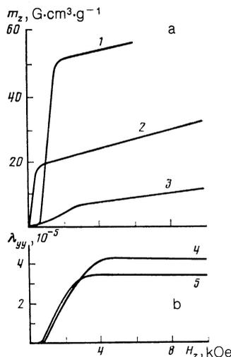
FIG. 2. Isotherms of the magnetization (a) and the magnetostriction (b) in  $\mathbf{H} \parallel \mathbf{c}$ : 1), 5)  $T = 4.2$  K; 2) 10.6 K; 3) 25.6 K; 4)  $T = 1.5$  K.
