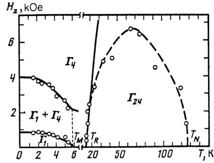
FIG. 3. Phase ( $H_z$ - $T$ ) diagram for the composition with  $\kappa = 0.3$ . The continuous curves are calculated; the circles and the dashed line are the experimental results; the dotted line represents the position of  $T_M$ .
