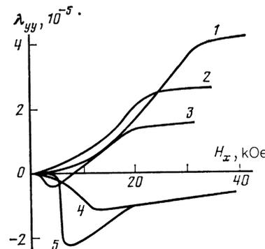
FIG. 4. Isotherm of the magnetostriction of  $\text{Dy}_{0.3}\text{Er}_{0.7}\text{CrO}_3$  in  $\mathbf{H} \parallel \mathbf{a}$ : 1)  $T = 1.5$  K; 2) 5.4 K; 3) 5.9 K; 4) 7.1 K; 5) 6.1 K.
