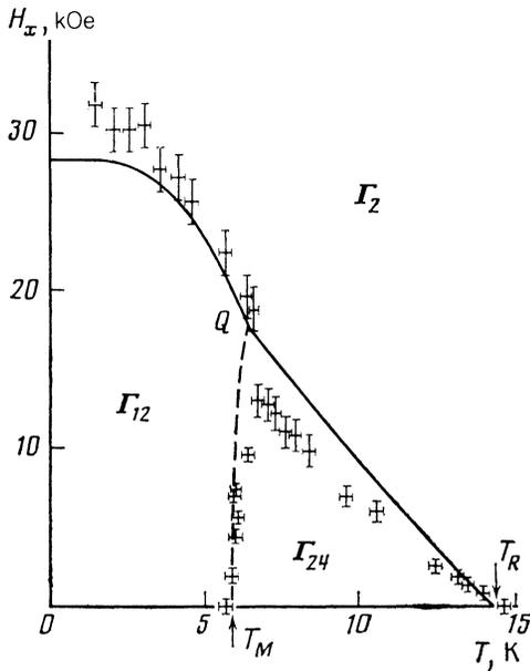
FIG. 5. Phase ( $H_x$ - $T$ ) diagram of  $\text{Dy}_{0.3}\text{Er}_{0.7}\text{CrO}_3$ . The points are the experimental values, whereas the continuous and dashed curves are calculated (the continuous curves correspond to a second-order phase transition and the dashed line corresponds to a first-order transition);  $Q$  is the bicritical point.
