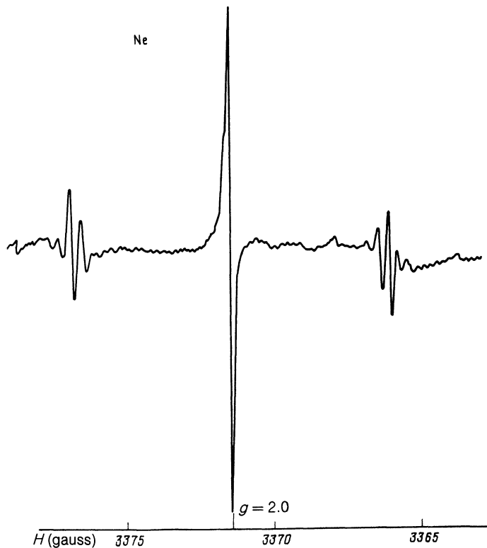
FIG. 6. ESR spectrum of short-lived paramagnetic centers in the neon cryocrystal with changes in the satellite lines; T = 4.2 K, Q = 4 mmole/h, f_{\text{res}} = 9437.39 MHz.
