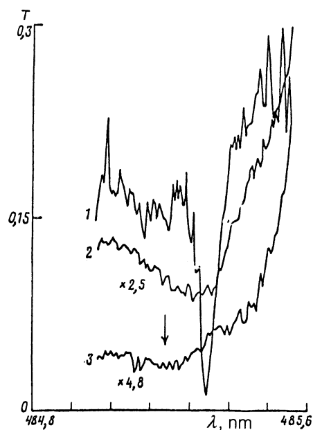
FIG. 8. Transmission spectrum of the mixed mode for maximum pumping: (2) 0.5 I_0 , (3) I_0 . For comparison we show the spectrum (1) for 0.05 I_0 , where I_0 = 3 to 5 \text{ MW/cm}^2 . A distinct violet shift of the exciton term is seen.
