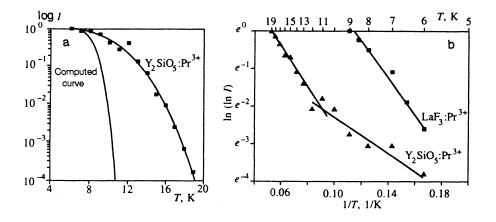
FIG. 4. Temperature decay of the amplitude of a photon echo in  $Y_2SiO_5$ :  $Pr^{+3}$  and  $LaF_3$ :  $Pr^{+3}$  crystals.
