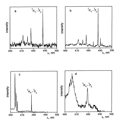
FIG. 1. Absorption spectra of a  $Pr^{+3}$  ion in the region of the resonant transition  ${}^{3}H_{4} \leftrightarrow {}^{3}P_{0}$  at temperatures of 1.5 K (a, c) and 77 K (b, d) for Y<sub>2</sub>SiO<sub>5</sub>:Pr<sup>+3</sup> crystals (a, b) and LaF<sub>3</sub>:Pr<sup>+3</sup> crystals (c, d).
