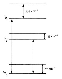
FIG. 3. Simplified energy-level scheme of a  $Pr^{+3}$  ion.
