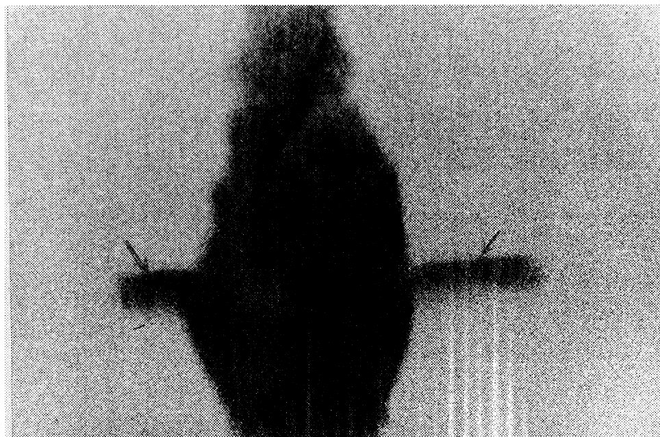
FIG. 2. Side view of the “jelly” formed around the cathode and within the anode ring. The anode ring is identified by the arrows.
