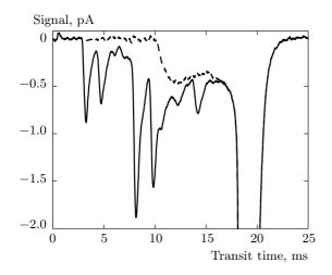
Fig.1. Results from a time-of-flight mobility experiment performed at 0.991 K as reported in Ref. [22]. The solid curve shows the signal arriving at the collector as a function of time. The dashed curve is the signal after an algorithm has been used to remove the peaks. The length of the experimental cell is 6.15 cm and the drift field is 82.1 V cm<sup>-1</sup>
