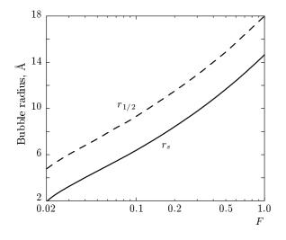
Fig. 3. Bubble radius on the fission model as a function of the fraction F defined in the text ( $r_s$  is the radius at which the helium density first becomes nonzero and  $r_{1/2}$  is the radius at which the density equals half of the bulk density)
