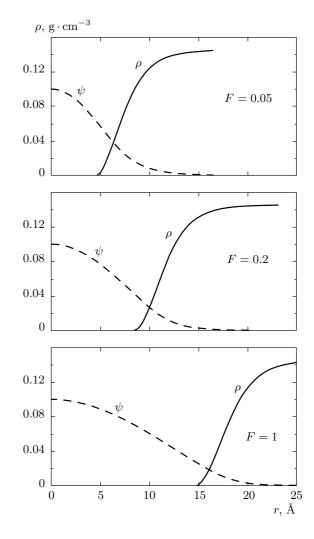
Fig.4. Helium density profile  $\rho(r)$  and the electron wave function  $\psi(r)$  for different values of the fraction F discussed in the text. In each part of the figure, the wave function  $\psi$  has been scaled to have the value 0.1 at the origin
