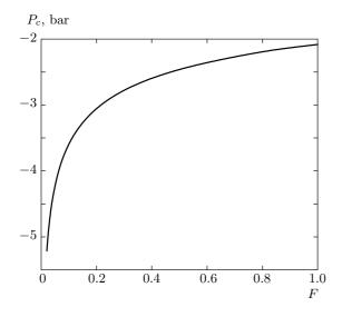
**Fig. 6.** Critical pressure  $P_c$  at which a bubble explodes as a function of the fraction F defined in the text
